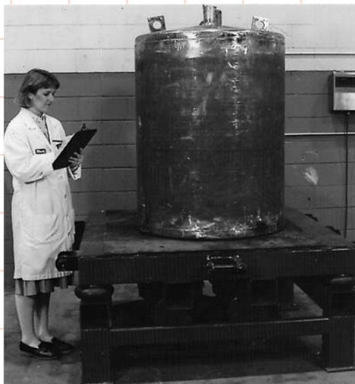
Vibrating table used to test density and material weight for each load. Table also tested for weldment cracks and fatigues during a normal 24 hour test cycle.
