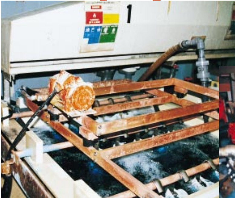
Model 2P-100CE mounted to top of specially designed rack holder. Racks for PC-boards were put into tank by hand.
