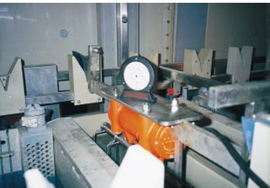
Model 2P-150CE used on single rack design for rinse cycle after PC-Board drilling. 100% of drill burrs are removed.
