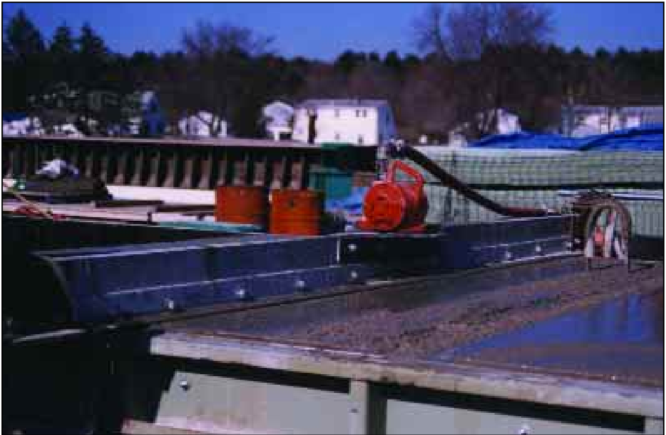
Model CCF-5000 Silent Pneumatic Vibrator on 10 ft. screed.
