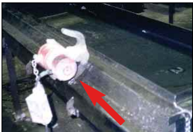
Model US-450 on wedge-bracket for vibrating lid on burial vault form.
