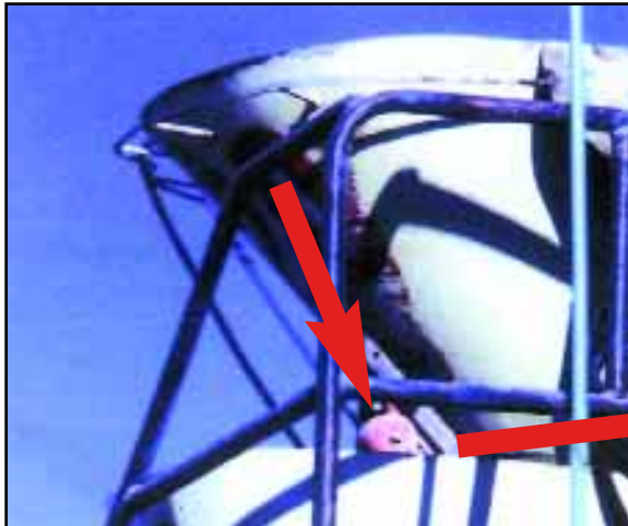
VIBCO VS-250 air vibrator mounted on the charge hopper of a front discharge mixer truck. (Complete kit available.)
