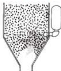
BRIDGING material hanging at lower slope.
